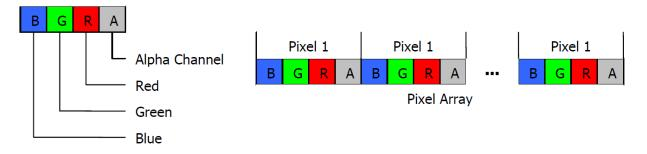
Each of the bytes in the RGB quad specify the intensity of the given color. The value ranges from 0 (the darkest color value) to 255 (brightest color value)
